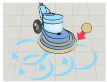
6 When dry, buff to a shine using 7 Let surface dry. appropriate coloured pad and machine.
