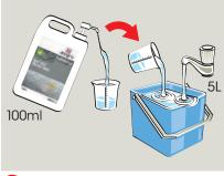
4 Dilute 100ml of solution per 5 litres of water in a bucket.
